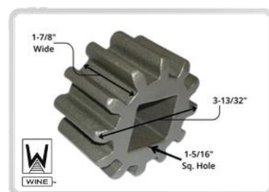
DA Pt # DA-70209 Alt Pt # DA-29-A Description: Pinion Gear, 1-5/16" Sq. Hole, 1-7/8" W
